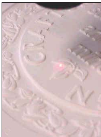
The Renishaw Cyclone system (left, right and below right) digitizes plaster and other models with a laser probe attached to a precision coordinate measuring machine (CMM). You can see the bright spot of laser light in the lower photo.
