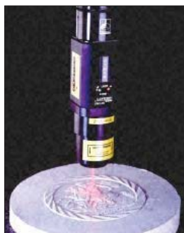
The Renishaw Cyclone system (left, right and below right) digitizes plaster and other models with a laser probe attached to a precision coordinate measuring machine (CMM). You can see the bright spot of laser light in the lower photo.
