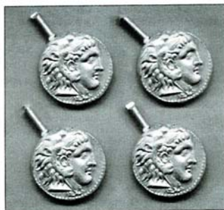
These four castings were made using an identical genuine coin as a master. Note that they all share identical features which distinguish them as originating from that same coin. (The casting sprues have not yet been removed from these coins.)
